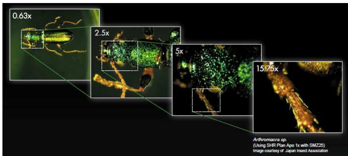
**Auto Link Zoom (ALZ):** Provides seamless viewing at different magnifications: By adjusting the zoom factor ALZ maintains the same field of view when switching objective lenses
