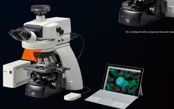
The dedicated, simple remote control pad allows motorized changing of objectives and filter cubes, and shutter operation
