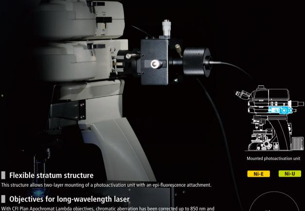
With CFI Plan Apochromat Lambda objectives, chromatic aberration has been corrected up to 850 nm and transmission improved in the long wavelength range, increasing accuracy and efficiency of laser excitation at target site.
