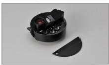
Motorized excitation filter wheel (Ni-E) Excitation filter positions (8 positions—using 25mm filters) can be changed at a high speed of 0.15 sec. between adjacent positions.
